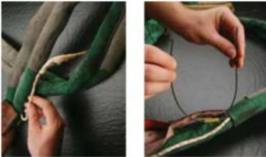
External indicators have been added in attempts to provide signs of core wear or damage. **The common result of each piece of this sling jewelry is the removal of the sling from service** and its return to a manufacturer for evaluation. The load bearing core, with certain rated capacities, remains hidden. Training for external indicators is confusing and costly and held outside the scope of standardization.
