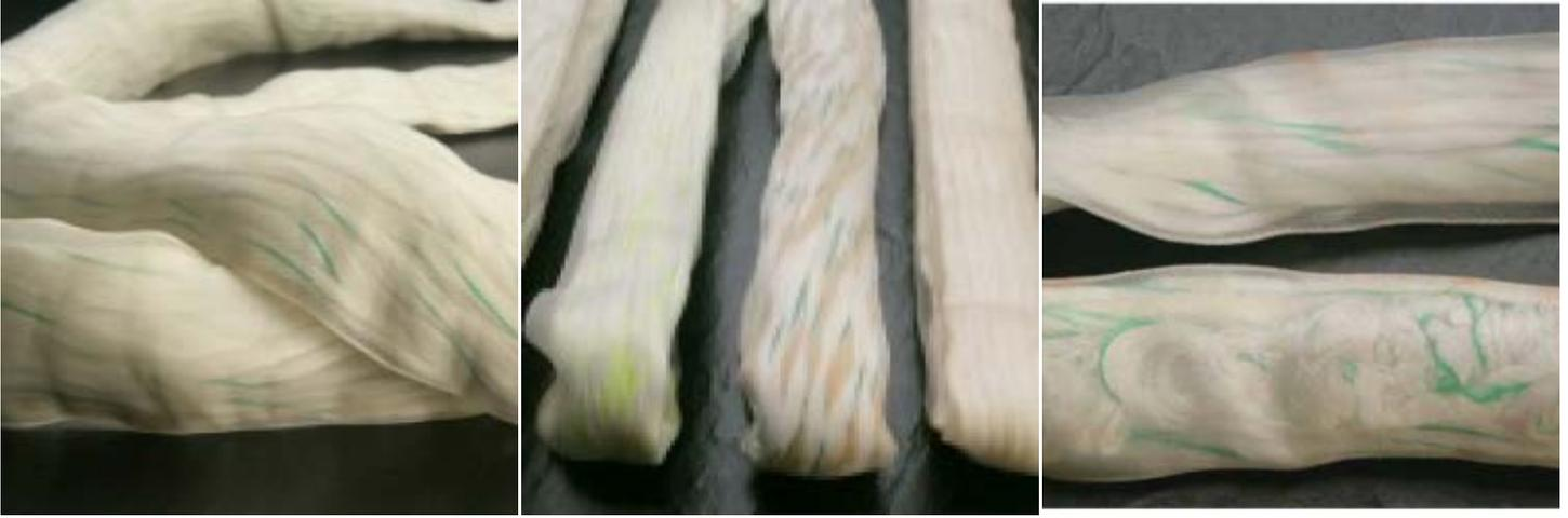
The transparent cover embodies and protects without prohibiting a visual inspection of the working roundsling, the core, or the lifting sling!
